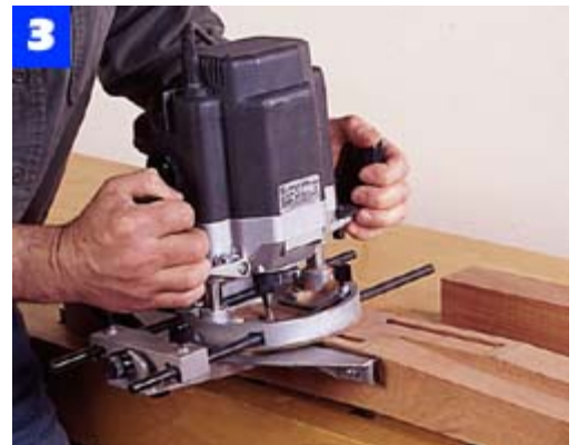
Rout the leg mortises with a spiral up-cutting bit. Another leg helps support the router while making these cuts.
