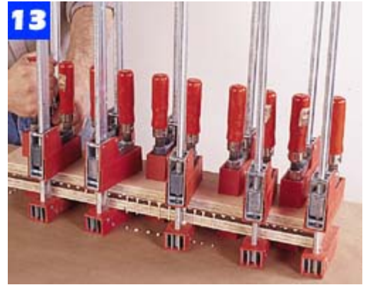
Starting at the center, apply clamps along the panel. A modest amount of glue will squeeze out along the edges.
