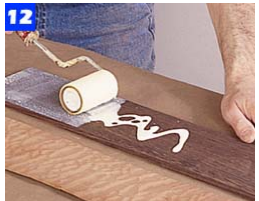
12 Use a foam roller to spread glue on the wenge panel. The glue must cover the surface, but shouldn't pool.
