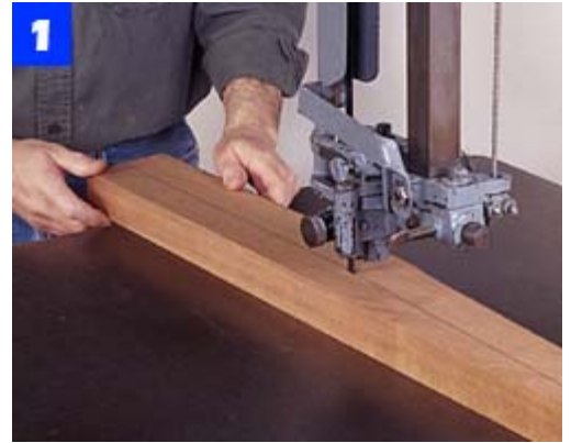
Use a band saw to cut the rear leg shapes. Keep the saw kerf on the waste side of the layout line while cutting.
