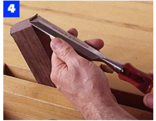
Use a chisel to cut a 1/4-in. bevel at the top end of a wenge blank. Then, cut a leg cap from the blank.
