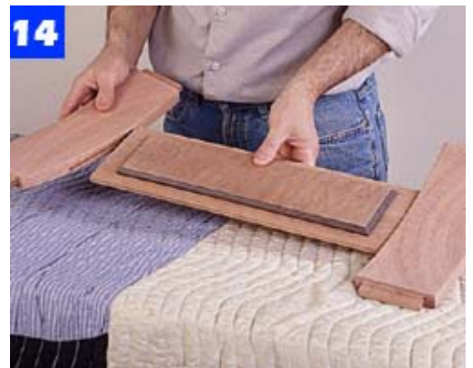
Begin assembly by joining the splat to the back rails. You don't need to use glue unless the joints are loose.
