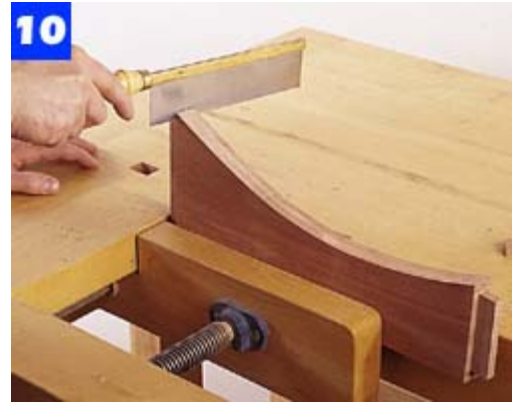
10 Clamp a side rail in your vise and use a dovetail saw to cut the shoulders at the top and bottom ends of each tenon.
